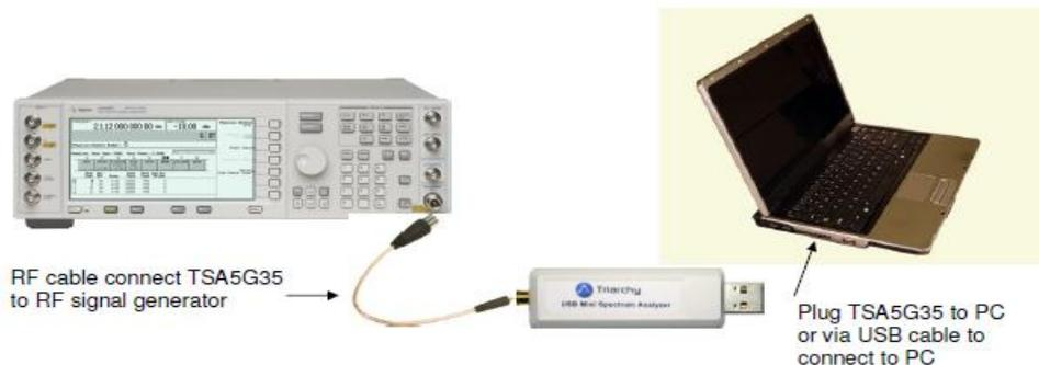
**Figure 9 System Connection**
