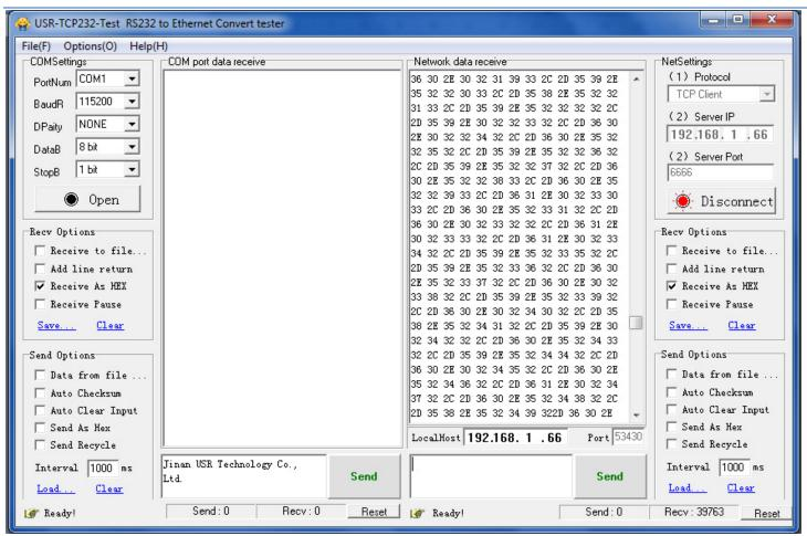
You can input \$Stop, then click send data key. The UsbApp will execute command to stop the scan, you also can send Start command with different setting to implement measurement, the receive data window will show all the data of measurement.
