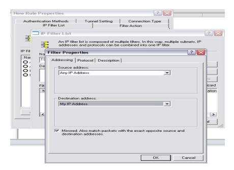
In the Filter properties and protocol item, mark From this port and input 6666 (inbound), mark the To this port and input 6666 (outbound), click OK key after setting.
