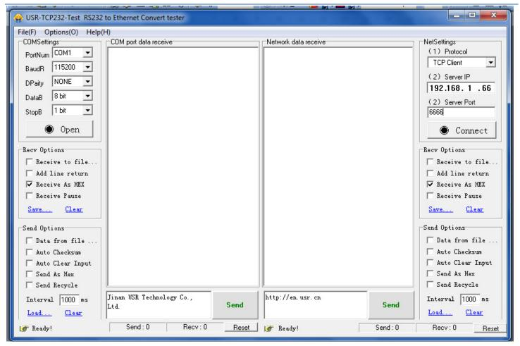
USR\_TCP232 Tester has network monitor and Com port monitor (USR-TCP232-Test.exe). Only the network monitor will be used in this case. First, setup Network Settings: select "TCP Client" in (1)Protocol window, input IP address in (2) Server IP window, input 6666 in the (2) Server Port window.
