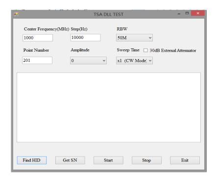
Please plug the TSA series Dongle into the PC, and click the Find HID to send setup command. The USB HID link will setup and handle data will show up:
