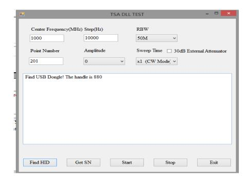
Click Get SN key, the SN command will send to Dongle and SN number will show on the window. please note, the calibation file must match with your dongle, otherwise, the program will not work.
