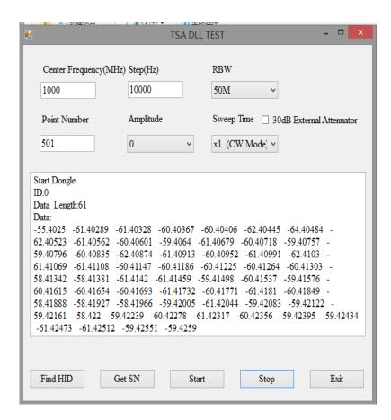
You can find data.txt file, change this log file name into data.csv, and open it by excel. Just keep one frame data, for this case the 501 point data, then show date with image. You can find signal waveform which will be exactly same as TSA program.
