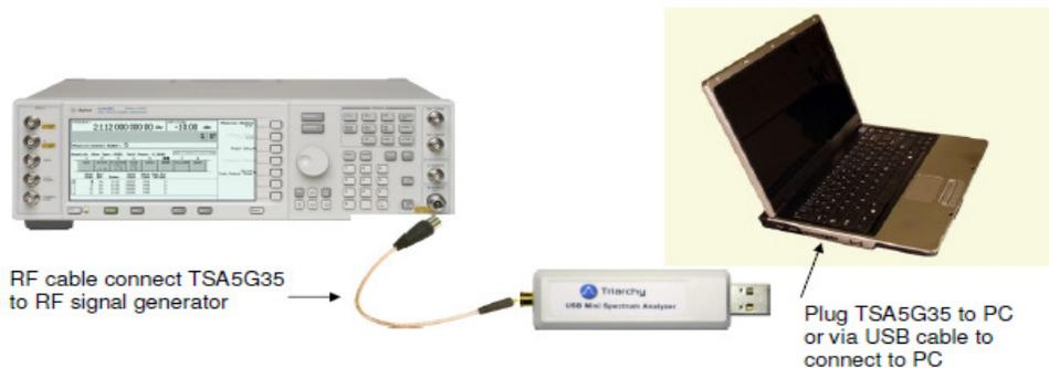
**Figure 9 System Connection**
